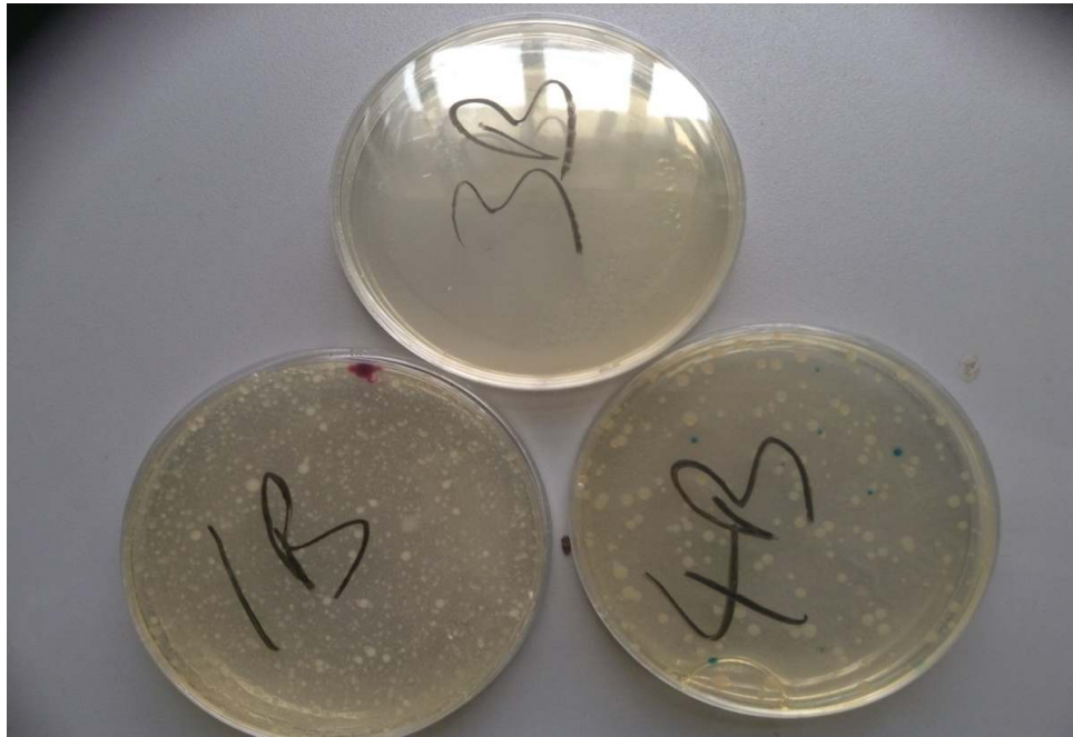
Fig. 1. Total and fecal coliform count tests, showing the blue and pink colonies
