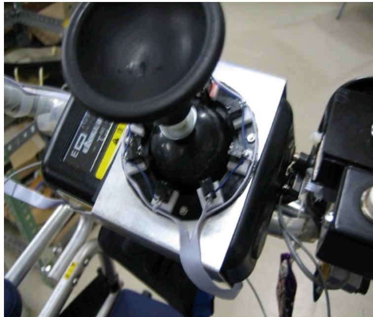
Figure 8. Joystick with eight limit-switches.
