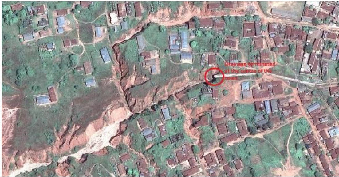
Fig. 4. Synoptic view from remote sensed data showing termination of drainage at the center of the town (Source: [25])
