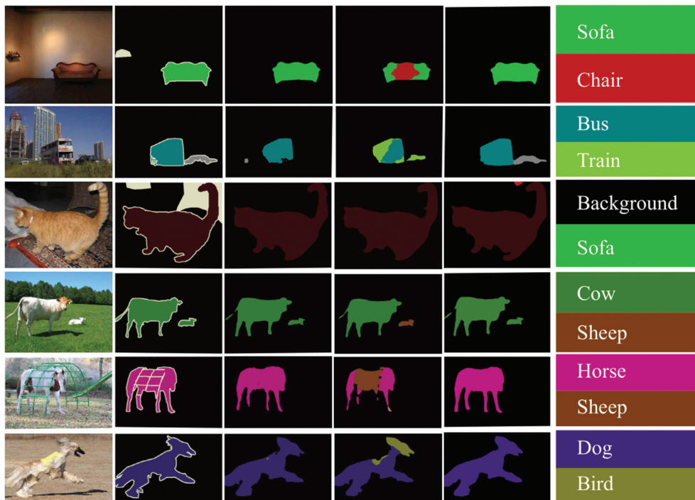
Figure 4. Visual improvements on PASCAL VOC 2012. From left to right are images, ground truth, predictions of PSPNet, UPerNet and DSPNet, respectively. It shows that DSPNet can both suppress the intra-class inconsistent segmentation and improve the quality of boundary.
