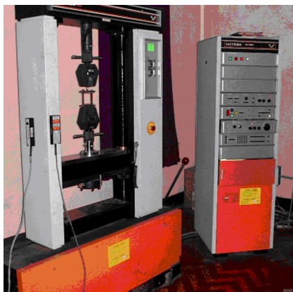
Fig. 2. Adhesion test set up Instron 1195
