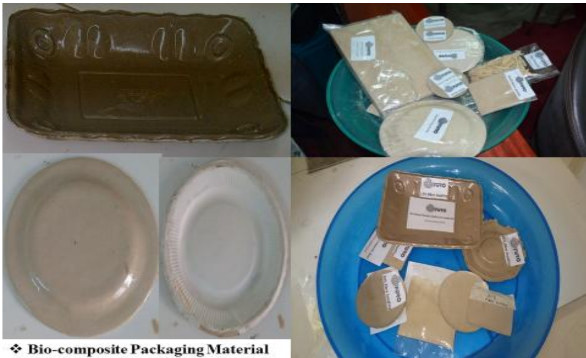
Fig. 2. Fabricated prototype packaging material by hand layup contact molding technique
