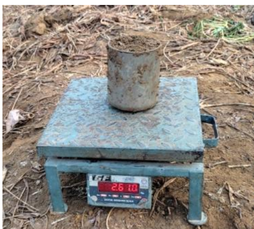
Fig. 1. Measurement of mass of soil contained in core sample
