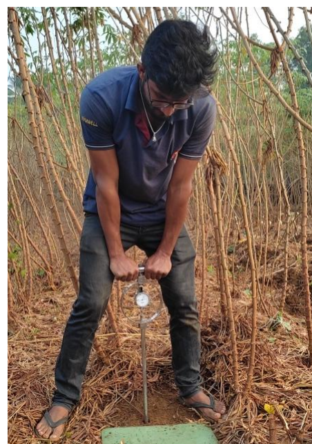
Fig. 2. Determination of soil cone index
