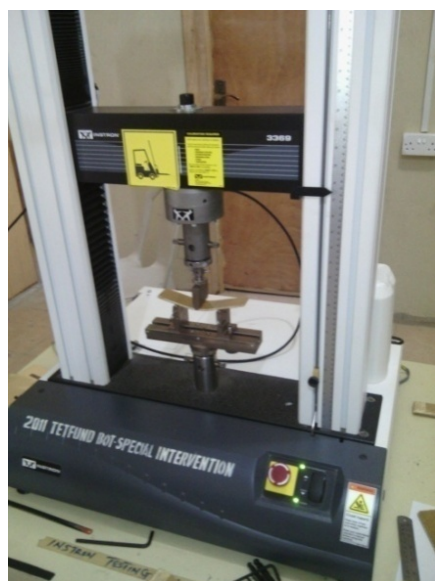
Figure 6. UTS machine sample loaded for flexural testing.
