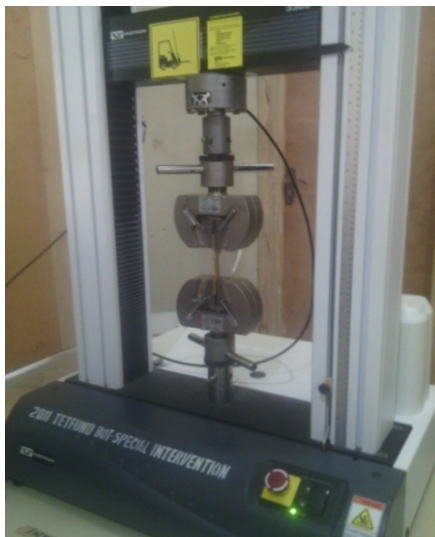
Figure 5. UTS machine sample loaded for tensile testing.
